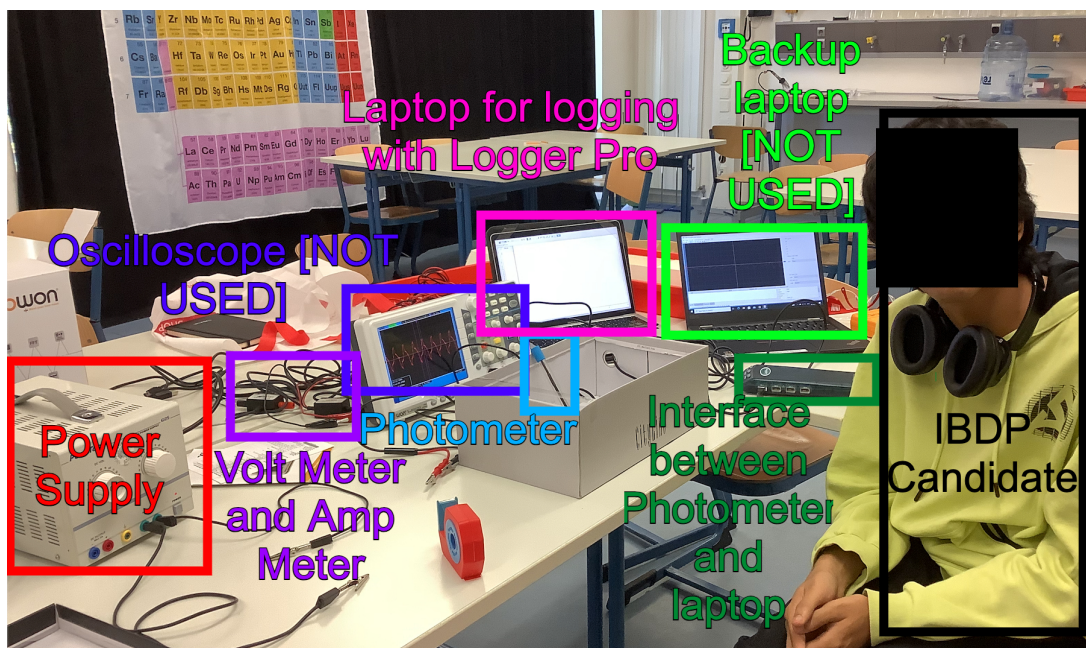
Figure 4: Photo of the setup, on the day of the experiment (IBDPCandidate)
